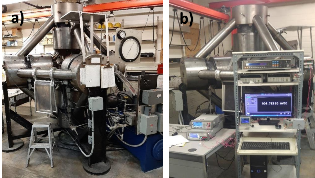
Figure 2.1a (left): An image of the 1000-ton cubic anvil press. Figure 2.1b (right): Experimental set-up: a DC current source and a multimeter are connected to the press, with a computer to read and display measured values.
