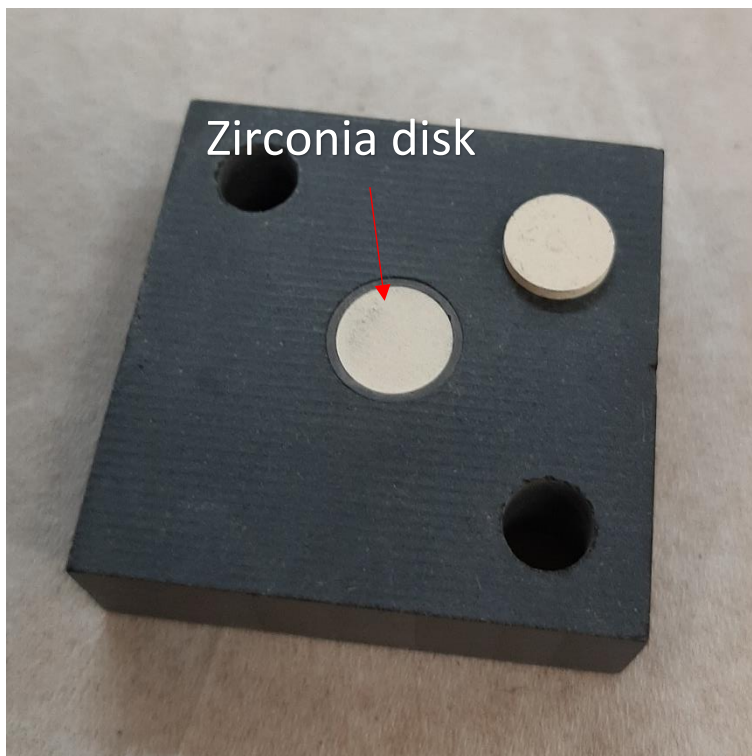
Figure 2.9: end section of the cell with the zirconia disk to improve containment.
